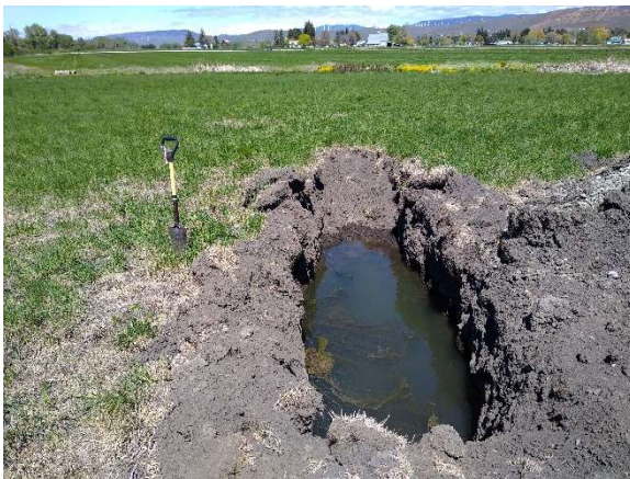
Photo 11 Test pit with groundwater at 3 ft. View toward NE.
